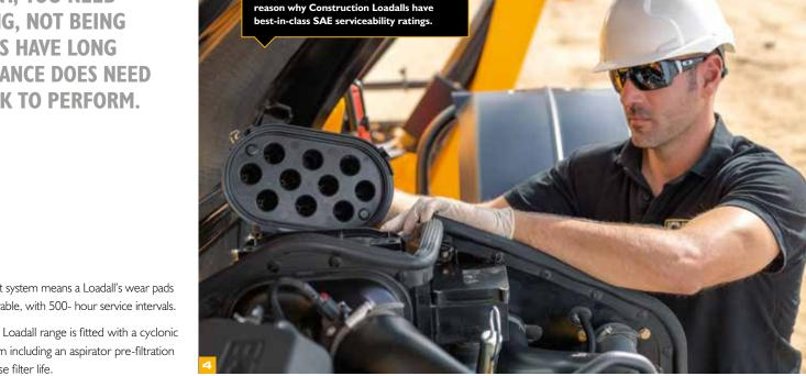
The filters on a Loadall (engine oil, hydraulic oil and fuel) are centrally located for fast, easy servicing. The air filter double element
