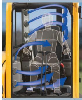
Heating and air conditioning keeps operator comfortable.
